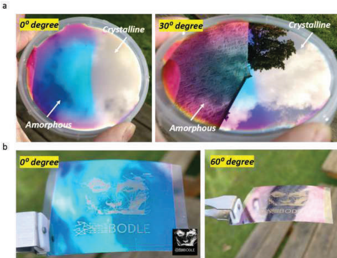
Figure 5 – A prototype SOVD film showing both angle dependence and a large colour contrast between the amorphous and crystalline phases. a. An angle dependent SOVD film is deposited on a glass wafer and partially switched to the crystalline phase by carefully positioning half of the sample on a hot plate set at 250° C. No roughening of the surface is visible as expected from a purely phase change driven induced colour contrast. b. A film with identical optical design is deposited on a PET film and switched using a continuous, rastering type visible laser system. The expected phase change induced colour contrast is followed by a small increase in roughness of the plastic film. This is attributed to a softening of the substrate induced by laser overheating. Substituting the continuous laser system with a pulsed system approach is expected to eliminate this issue without lowering the degree of colour contrast. This is due to extremely fast crystallization dynamics of the PCM that requires a few tens of nanoseconds to fully crystallise.
